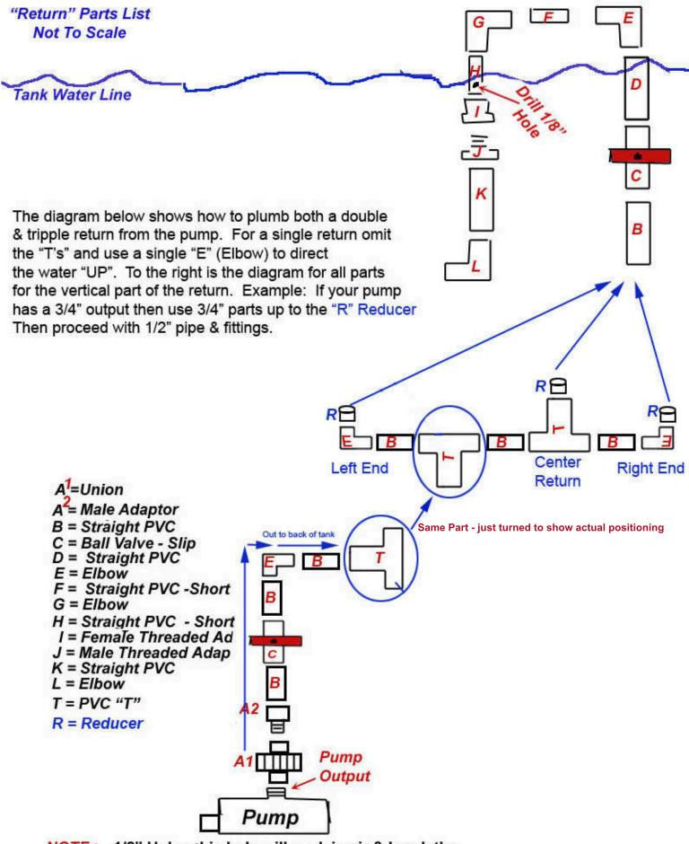
NOTE: 1/8" Hole - this hole will suck in air & break the back feed upon turning off the pump or for a power outtage. Keep this hole clean or your return will continue to siphon water to your sump until the bottom elbow (L) sucks air!
